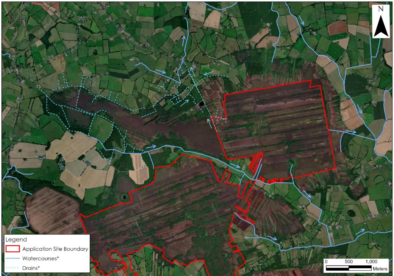
Figure 9-4: True Drainage of Lisclogher Bog Based on Site Walkovers and Lidar Data
